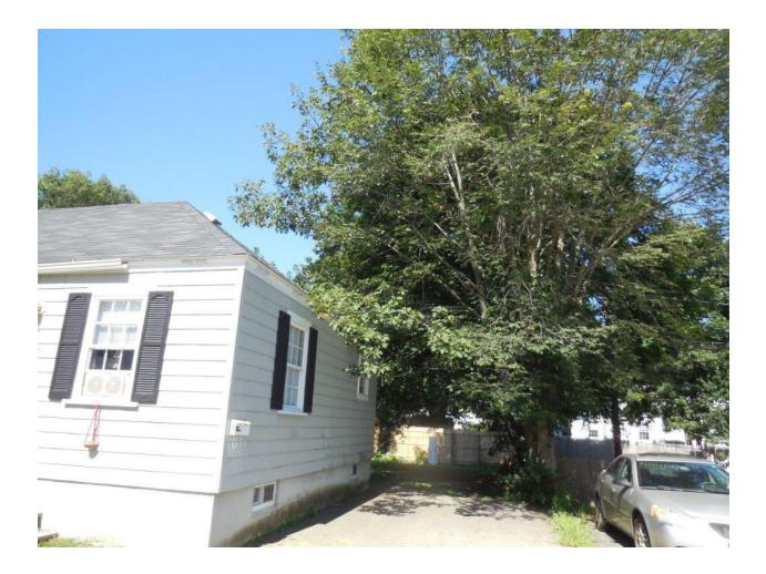
UPCS Inspectable Area: Site: Grounds: A tree is contacting the roof of the building. Level 2 (Level 3 for more extensive contact/damage).
