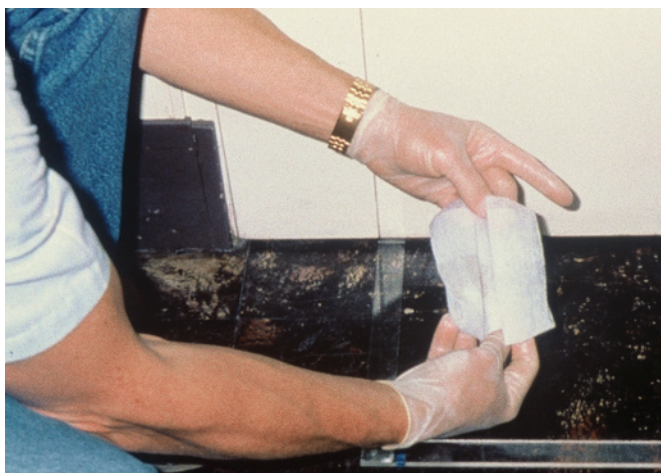
FIGURE 5.11d Folding wipe over for second pass.
