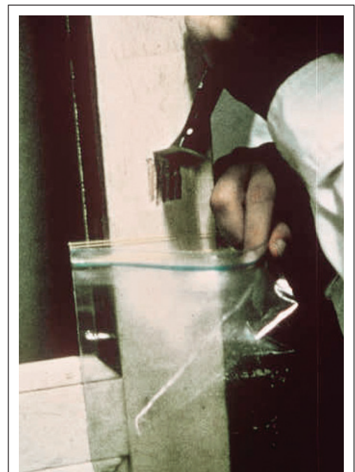
FIGURE 7.5 Removing paint-chip sample.
